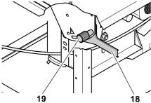
In order for the blade angle not to change during cutting, the blade is locked in position with the turning knob (19).
